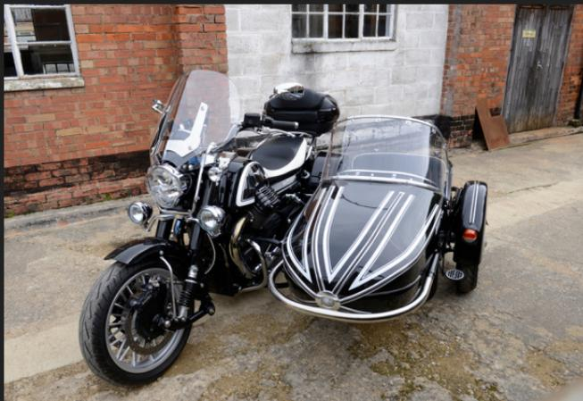
The GP700 is the wide bodied version of the GP sidecar (overall width 40"/1010mm). It seats an adult and child or two children, while retaining the classic looks of the other GP models. Its bench seat is 700mm (27.5") wide at hip height. This sidecar is suitable for compatible motorcycles over 500cc.
